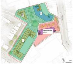
Figure 10.4.2 Indicative construction sequence for the Wood Green Library Site including meanwhile use location.
